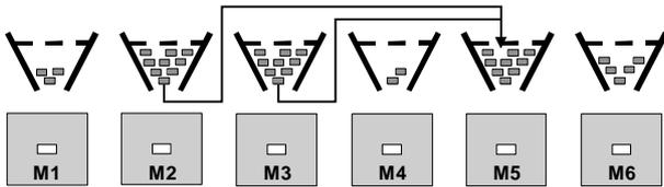
Fig. 8: Virtual buffers as a network of funnels.
