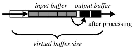
Fig. 5: Virtual buffer of a machine.
