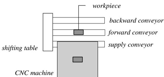
Fig. 3: System components.
