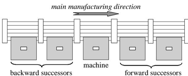
Fig. 6: Forward and backward successors of a machine.
