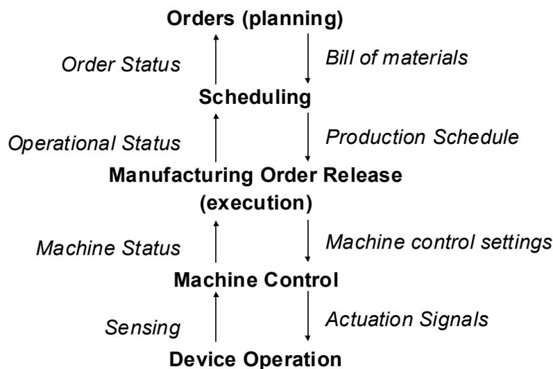
Figure 7 Typical Manufacturing Control Hierarchy
