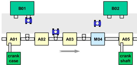
Fig. 2: Introduction of flexible buffers (phase 1).
