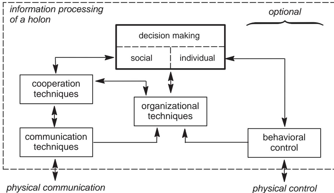
Figure 5: Agent-oriented architecture for a holon.
