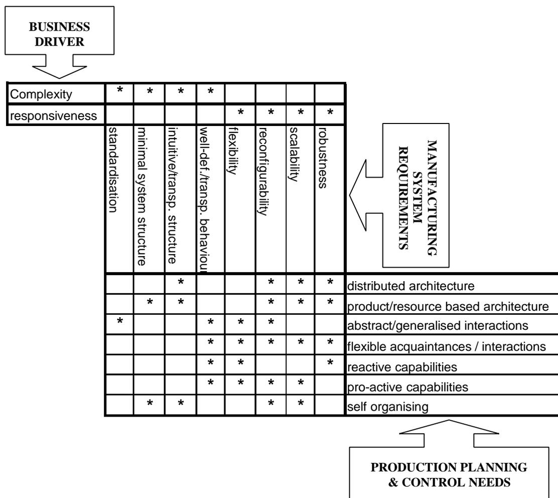
**Figure 3 Additional Production Planning and Control Needs [66]**
